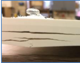
Figure 6: Risk of splicing when screwing without pre-drilling
